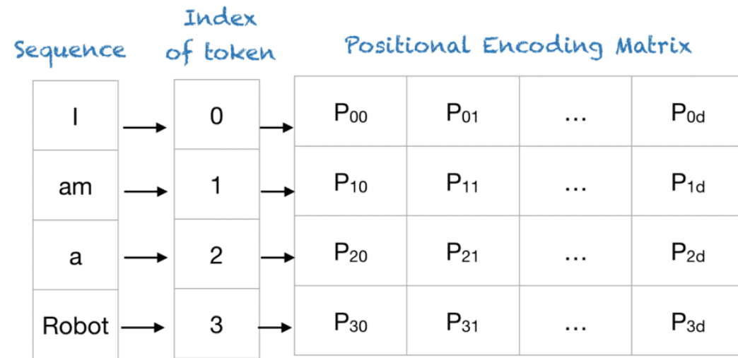
Positional Encoding Matrix for the sequence 'I am a robot'
